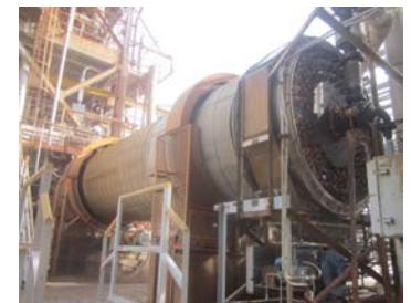
8'0"x40'0" Steam Tube Dryer #104443
