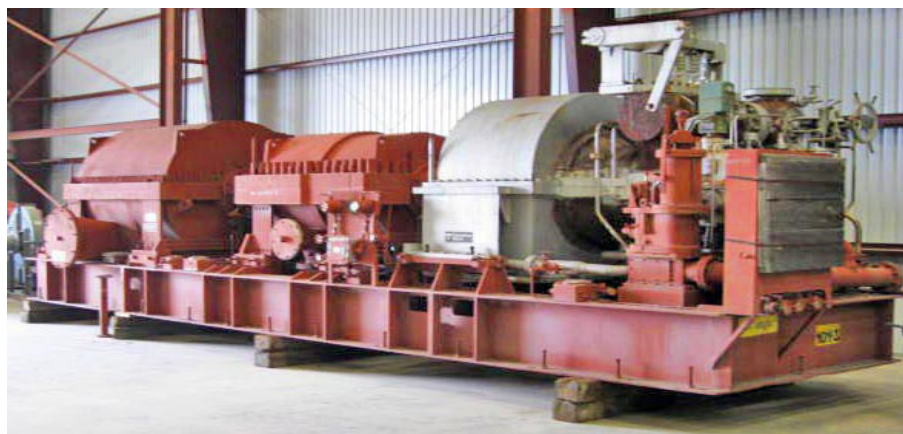
Photo Above: Complete 101 Air Compressor Train
