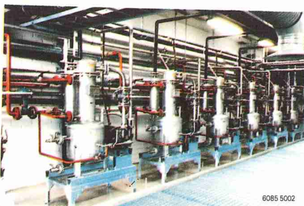
10 APOVAC units installed in a separate room of a fine chemicals plant.
